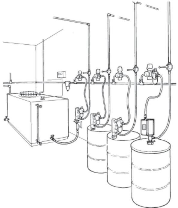
For environmental and stock control reasons all lubricants should be stored in a separate room. The drawing above shows a typical layout. High consumption oils should preferably be stocked in tanks with the pump being either wall or floor mounted. The prime consideration regarding the storage of grease should be to prevent any risk of contamination from entering the drum since this will ultimately find its way into the components being greased.
