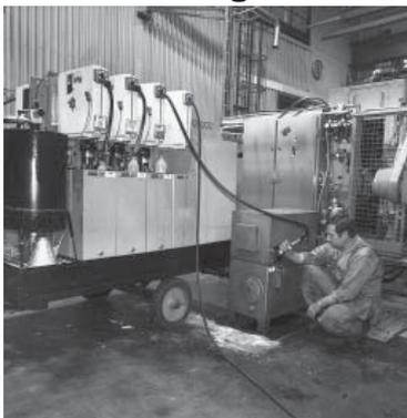
*The hose reels provide a working radius of approx. 10 meter and make it easy to dispense lubrication oil even where space is restricted. OriPac has a built-in oil filter that guarantees absolutely clean lubrication oil.*
